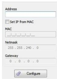
In the **IP Address** field, enter the IP address being configured; do the same with the **Netmask** and the **Gateway** if necessary. After entering the device configuration, press **"Configure"** to send the configuration to the unit.
